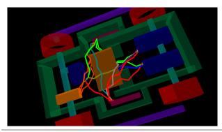
**Figure 11.** ProtoSim is a robust, extensible simulator for Proto agents. In this example, Proto is being used to semi-automatically wire the internal components of a robot.
