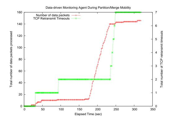
Figure 5.16: Network statistics collected by the data-driven monitoring agent during the partition/merge mobility scenario. During this scenario, failures in plan execution occurred due to lack of network connectivity.
