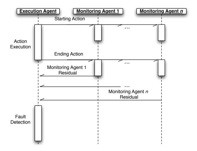
Figure 4.3: Sequence diagram showing the interaction between the execution agent and analytic monitoring agent(s).
