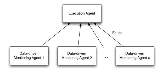
Figure 4.4: Flow diagram showing the interaction between the execution agent and datadriven monitoring agent(s).
