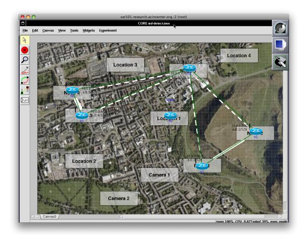
Figure 5.6: Screenshot of the IED detection scenario running in the network emulator, CORE. The blue circles are hosts in CORE and the green lines represent network links. The white rectangles in the background of CORE are used to show the starting locations of the hosts for the IED detection scenario.
