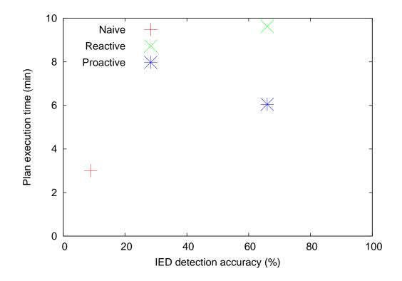
Figure 5.12: Mean IED detection accuracy versus mean plan execution time of the random planning agent in combination with each execution agent.
