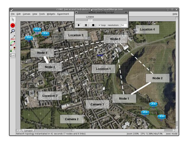
Figure 5.7: Screenshot of the partition/merge mobility model running in CORE. The blue circles are the CORE hosts, the white rectangles show the starting positions.
