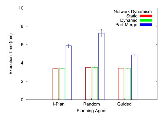
Figure 5.10: Mean plan execution time for plans that executed successfully to completion by planning agent and the network dynamism (as indicated by the mobility scenario). Static mobility exhibits the least network dynamism, dynamic has varying link weights but never completely partitions the network, and partition-merge (part-merge) separates the network into two islands and then merges the islands.
