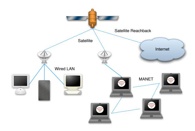
Figure 1.1: Example of a heterogeneous network. In this type of network, multiple different technologies (satellite communication, MANET, and wired Ethernet) are combined.
