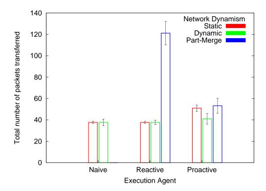
Figure 5.14: Average number of packets transmitted across the entire network for various execution agents under different network dynamics. The naïve execution agent never successfully completed executing a plan in the partition/merge mobility scenario, so it is not included in this figure.
