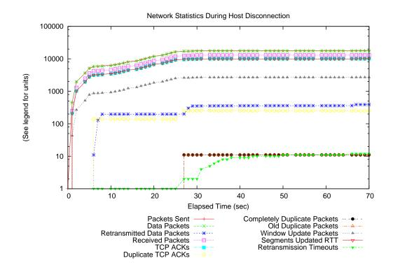
Figure 4.5: Graph illustrating the network criteria tested during the disconnection modeling process for the data-driven monitoring agent. A disconnection occurred roughly at the point on the graph where retransmission timeouts increases sharply.
