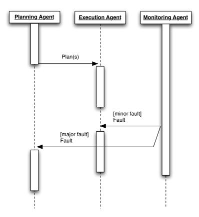
Figure 3.3: The sequence diagram for the plan execution process. The planning agent is responsible for creating plans and passing them to the execution agent. The execution agent invokes services on the hosts according to the plan. The monitoring agents report execution faults to the planning and execution agent as needed.
