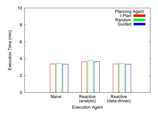
Figure 5.8: Mean plan execution times (in minutes) by plan, execution agent, and monitoring agent types. All agents and services are located on a single host so the network is not affecting the results.
