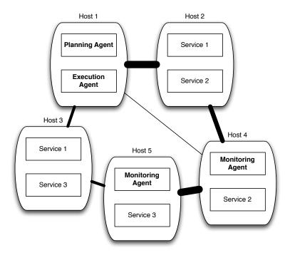
Figure 3.1: The conceptual diagram of the formal problem statement. Rounded rectangles represent hosts  $h \in H$ , which are capable of executing a set of services. Planning, execution, and monitoring agents reside on hosts. Lines between hosts represent communication links between the hosts and the thickness of the line is a representation of link quality,  $\omega_H$ .
