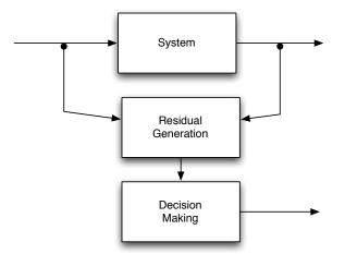
Figure 2.4: The main components of the analytical approach towards fault detection.
